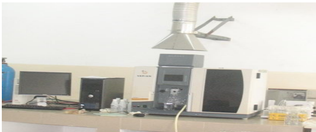
Plate1: VARIAN AA 240 Flame Atomic Absorption Spectrophotometer used for analysis of the fish samples
